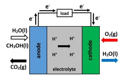
At the anode, methanol is oxidised.
