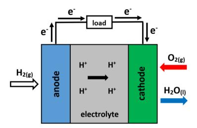
• At the anode, hydrogen is oxidised.
