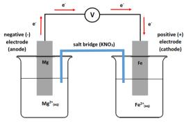
At the anode (oxidation):  $Mg(s) \rightarrow Mg^{2+}(aq) + 2e^{-}$ At the cathode (reduction):  $Fe^{2+}(aq) + 2e^{-} \rightarrow Fe(s)$ Overall reaction:  $Mg(s) + Fe^{2+}(aq) \rightarrow Mg^{2+}(aq) + Fe(s)$ Anions move in the salt bridge from cathode to anode. Cations move in the salt bridge from anode to cathode.
