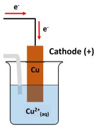
Electrons flow to the cathode from the anode. The  $Cu^{2+}(aq)$  ions undergo reduction.  $Cu^{2+}(aq) + 2e^{-} \rightarrow Cu(s)$
